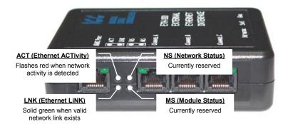
Figure 6: Module and Ethernet Indicators
